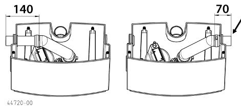
The pressure pipe is supplied ready mounted on the left-hand side. If the pressure pipe is required on the right-hand side, the section of pipe must be shortened by approx. 70 mm. If a ventilation pipe is not connected when the HEBEFIX EXTRA is connected directly, the left-hand side must be sealed from the inside with the sealing plug.
