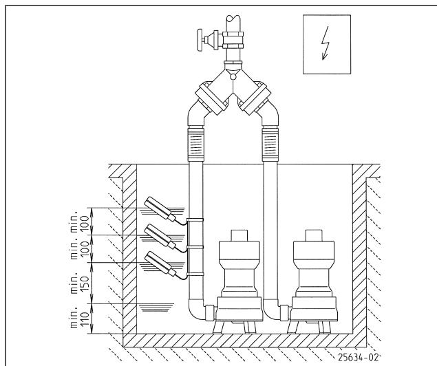
**Installation:** The submersible pump is fitted with a 90° connection and then lowered into the chamber or collecting pit using a chain.
