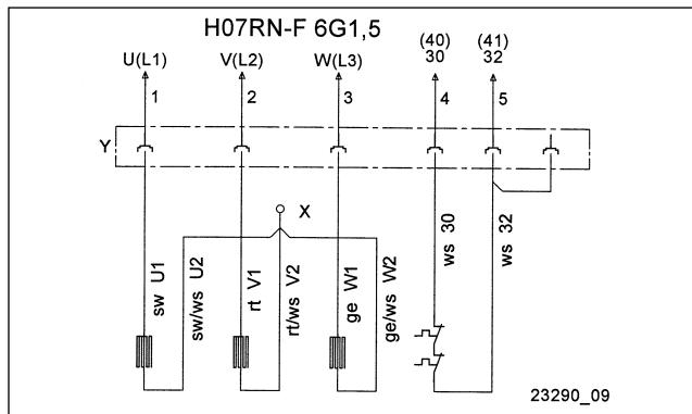
Alterations to the circuitry are to be made using crimp connectors (X) between the Coni plug connection (Y) and the built-in motor. The new crimp connection must be professionally made.
