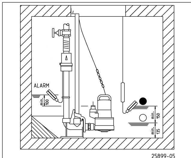
**Installation:** Fix the coupling base firmly to the floor of the collection chamber using wall plugs and then mount the guide rails. Next, install the pressure pipe including the necessary fittings, such as the non-return valve and shut-off valves.
