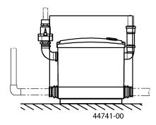
Before installing the system, secure the DN 50 connection sleeves to the inlet pipes with the clamps. Ensure a secure and tight fit!
