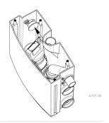
The on-site pressure pipe is connected to the HEBEFIX PLUS discharge branch with the arched discharge elbow. The maximum capacity specified by the manufacturer (see Technical data) must not be exceeded. Any deviations from this will impair the pumping performance.
