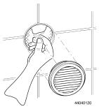
The supply package includes a round active carbon filter which minimises odours emitted into the room during ventilation. Maintenance and replacement work must be carried out from the outside through the ventilation grille.
