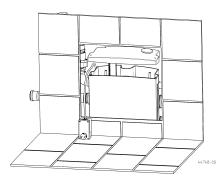
Loosen the four screws in the lid without removing them, and lift the lid off. The lid can now be put aside together with the plug unit.
