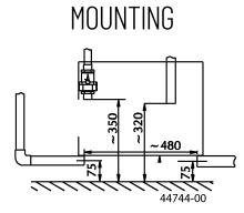
The inlet pipes, pressure pipe with the swing-type check valve and the ventilation are all mounted in the prepared installation space for the system.
