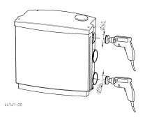
The pipe connections for the sanitary items to be discharged, such as shower, washbasin or household washing machine, must be opened with a hole saw and then deburred.
