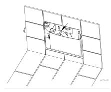
Loosen the wing bolt on the hose clamp on the discharge branch. The flexible discharge elbow can now be detached from the pressure pipe. Grip the pump by the handle and carefully take it out of the tank. Ensure that the float switch does not detach itself from the retaining brackets on the inside wall of the tank.
