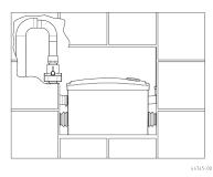
The pressure pipe must be laid without a gradient. If a gradient to the hand-over point is unavoidable, however, then a wider pipe with larger dimensions must be fitted after the highest point. This avoids a siphon which could result in malfunctions.
