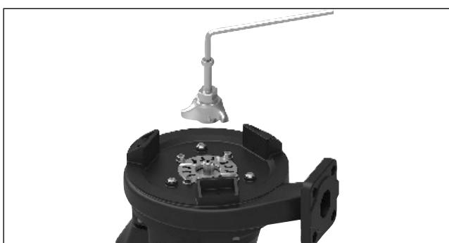
3. Unscrew the four hexagon socket screws on the top of the spiral housing, and take off the spiral housing.
