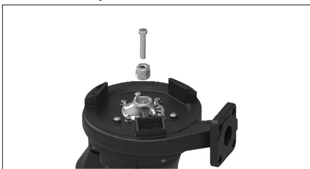
2. Remove the compression piece and screw the extraction tool (code no. JP50325) into the thread of the cutting rotor. Tightening the inner screw pulls the cutting rotor off the pump shaft.
