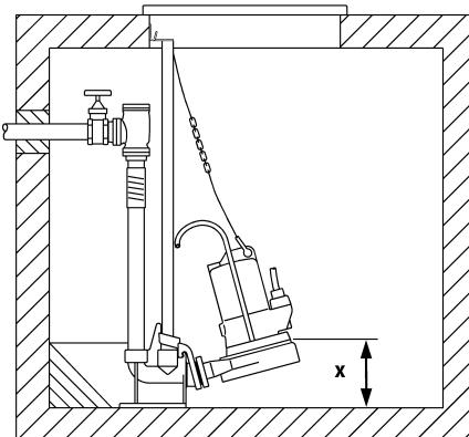
**Assembly:** Fix the coupling base firmly to the floor of the collection chamber using plugs and then mount the guide rails. Next, install the pressure pipe including the necessary fittings, such as the non-return valve and shut-off valves.
