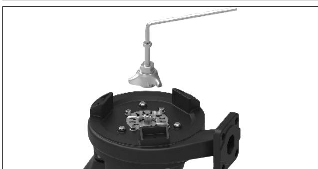
3. Unscrew the four hexagon socket screws on the top of the spiral housing, and take off the spiral housing.
