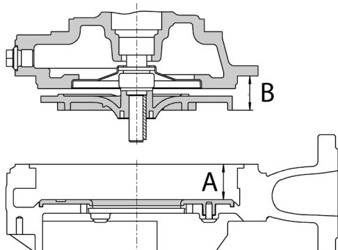
5. Measure dimension B on each blade and note the largest measurement.
