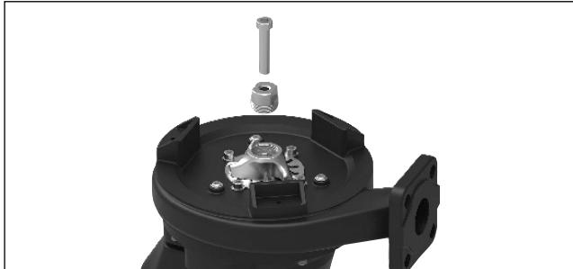
2. Remove the compression piece and screw the extraction tool (code no. JP50325) into the thread of the cutting rotor. Tightening the inner screw pulls the cutting rotor off the pump shaft..
