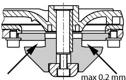
1. Block the cutting rotor with a piece of wood and unscrew the central hexagon socket screw.
