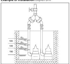
**NOTICE!** The floats of the level controller and alarm system are installed so that they are freely movable but not under the inlet. Please observe the minimum distances. The controls may only be installed in a dry and well ventilated room!
