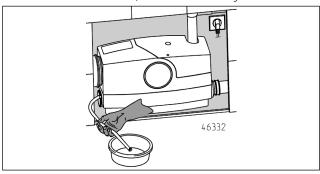
If a hose was fixed to the tank during installation, then the water in the system can be drained away quite simply through the hose and into a shallow container. The hose must then be resealed using a suitable stopper.
