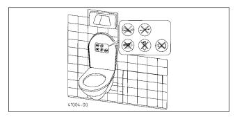
The sticker that is supplied with the unit and shows symbols giving instructions for use must be attached where it can be clearly seen by people using the toilet: for example above the toilet lid or on the inside of the lid.
