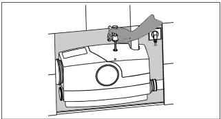
If the pump is sluggish or blocked, it can be set in motion again using a screwdriver, without any further disassembly. To do this, remove the stopper from the hole in the cover. Insert a long screwdriver (Torx 30 or grub-screw H5) through the hole in the cover. Turn the screwdriver gently until it engages with the slot in the motor shaft and then turn the shaft forcefully in both directions to clear the blockage.
