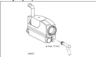
To drain the tank in an emergency, a section of garden hosepipe be connected to the tank at the bottom on the right-hand side. First, you will have to open up the 13-mm-diameter port by drilling through it with a spiral drill (maximum diameter: 9 mm). Push the hosepipe onto the port and secure it with a hose clip (tightening torque: 1.5 Nm). Make sure that the outlet opening of the hosepipe is securely sealed.
