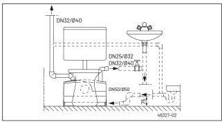
**NOTICE!** If a connecting pipe is fitted between the WCFIX and the toilet, this will result in malfunctions. This method of installation does not comply with the approval of the Deutsches Institut für Bautechnik (the German approval body for construction products and types of construction).
